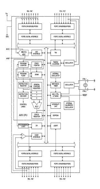
Fig 1. Internal Architecture of AVR Microcontroller
