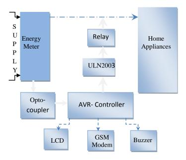
Fig 2. Circuit descriptions of AVR Microcontroller
